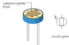
**Figure 4:** LDR as Fire Sensor
