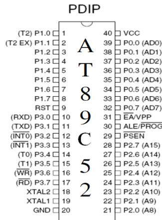
Figure 2: Pin Diagram of AT89C52
