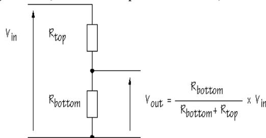
**Figure 5:** Voltage Divider Circuit
