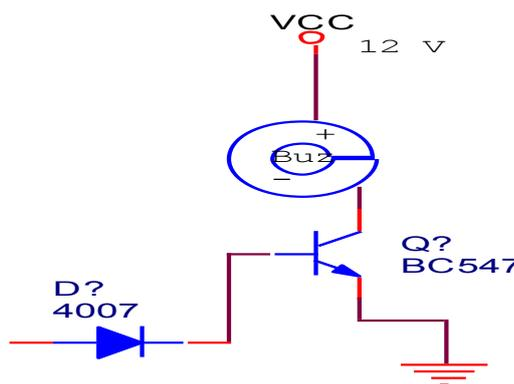
Figure 9: Buzzer driver
